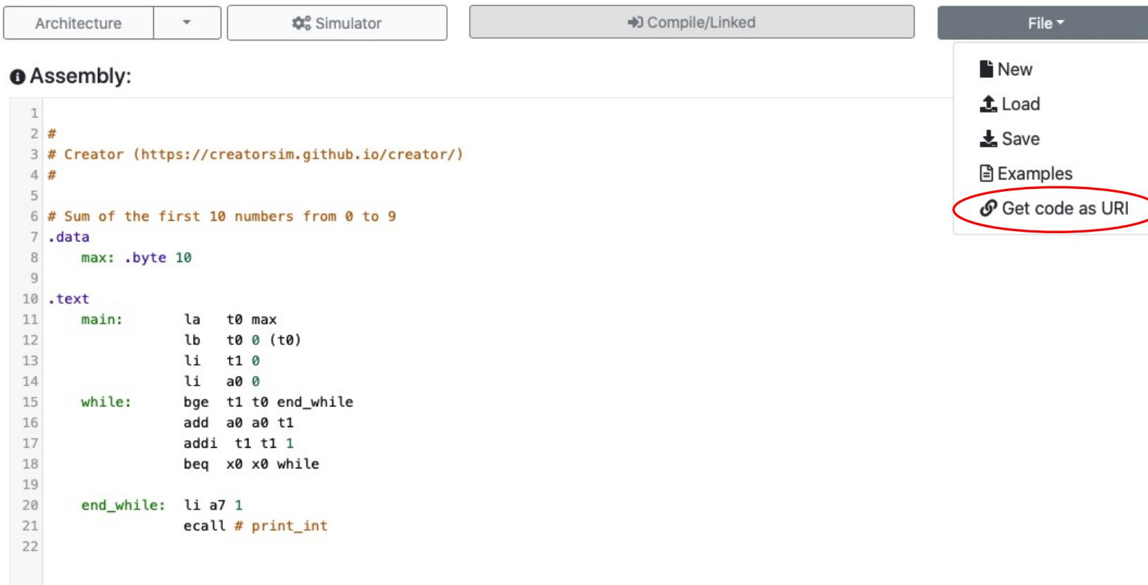
The screenshot shows the ARCOS assembly editor interface. At the top, there are tabs for "Architecture" (selected), "Simulator", "Compile/Linked" (disabled), and "File". The "File" menu is open, showing options: New, Load, Save, Examples, and Get code as URI, with the last option circled in red.
